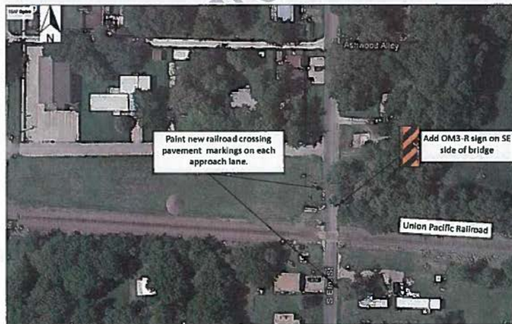
Figure 33 – Low-cost recommendations at UP Railroad & Elm Street crossing
