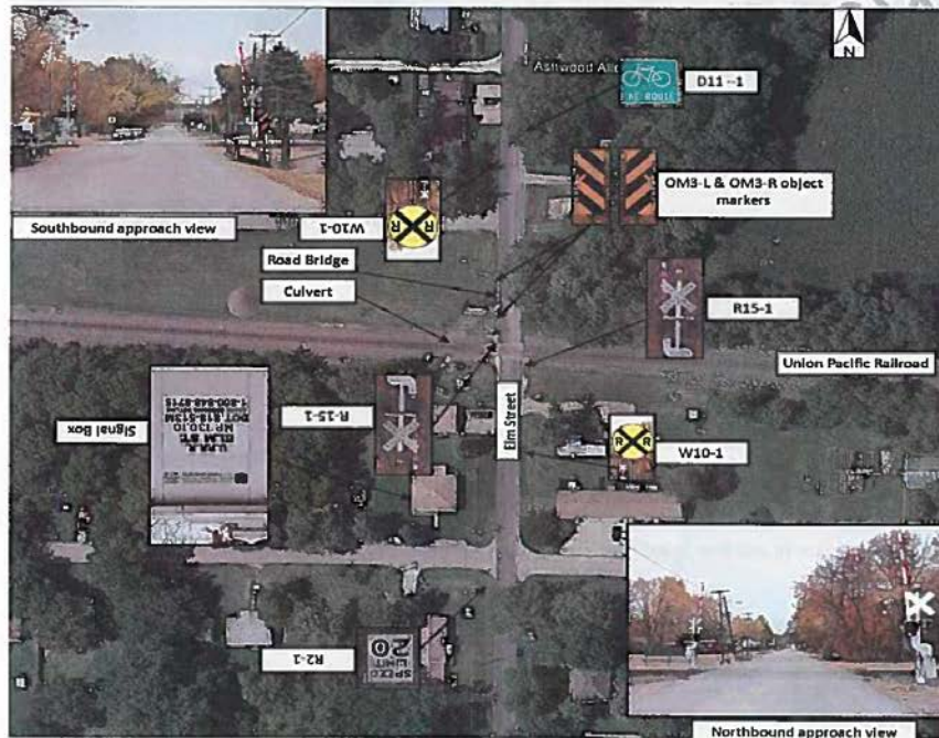
Figure 28 - Existing signs and pavement markings at UP Railroad & Elm location
