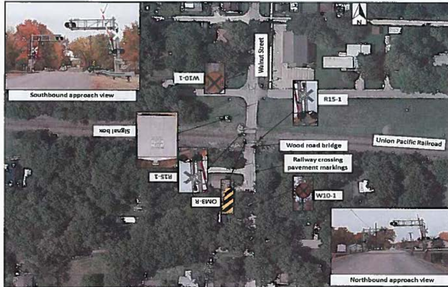
Figure 35 - Existing signs and pavement markings at UP Railroad & Walnut location
